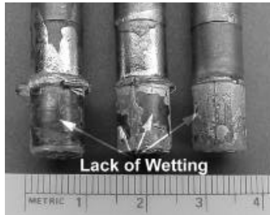
Figure 12. Examples of plugs that were not wet by the solder when spacing wires of nichrome were used.
