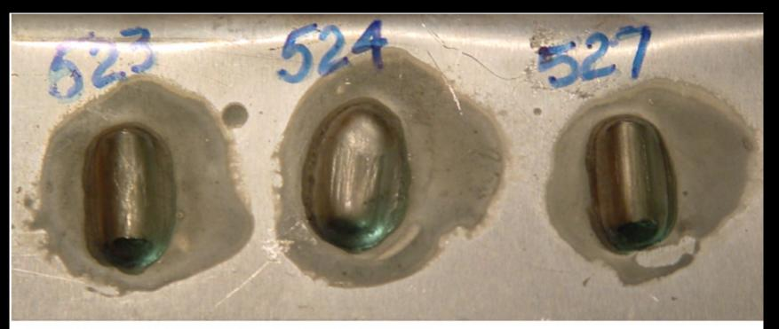
JOHNSON'S #523 LEAD-FREE SEMI SOLID BODY SOLDER ALLOY 82Sn/15Cu/3Zn, MELTING TEMPERATURE 428 - 940 F as determined by DTA at Ford Research Lab USED BY FORD AND OTHER AUTO ASSEMBLY PLANTS #524 EXPERIMENTAL SEMI SOLID BODY SOLDER ALLOY 85Sn/12.5Cu/2.5Zn, NARROWER MELTING RANGE Estimated 428 -880 F EXHIBITED MOST SLUMP OF THE SOLDERS TESTED #527 FORD BODY SOLDER
