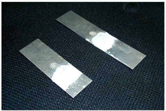
Figure 8. Ford specimens—soldered joint with solid solder.
