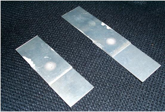
Figure 7. Ford specimens—reverse side shows what pre-soldered joint looks like.
